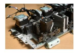
推针电机结构,有效缩短机头回转行程,功能更加稳定 Raising cam is controlled by motor,greatly reduce the carriage returning distance,function is more stable and effective
