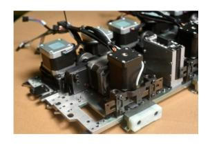
推针电机结构,有效缩短机头回转行程,功能更加稳定 Raising cam is controlled by motor,greatly reduce the carriage returning distance,function is more stable and effective
